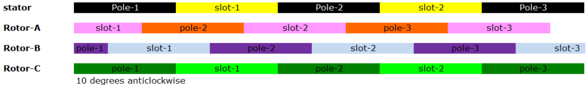
Fig. Operation of 3-stack stepper motor
