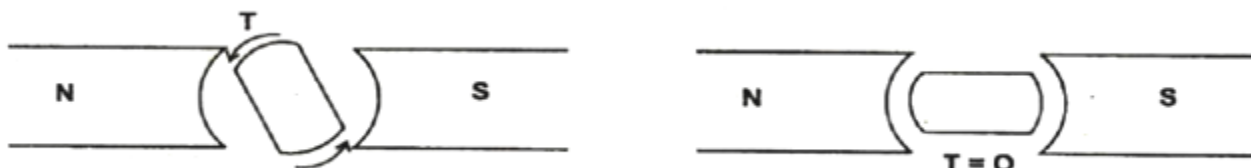
Fig. Rotor position due to revolving magnetic field
