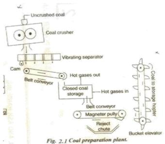
\* The coal preparation plant which include crushers, breakers, dryers, sizers and magnetic
