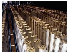
✤ The gas centrifuge process uses a large number of rotating cylinders in series and parallel formations.
