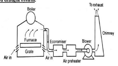
✤ In this system (ID fan) fan is located near the chimney base sure such that it draws the burnt gases form the furnace and bolus in to the chimney
