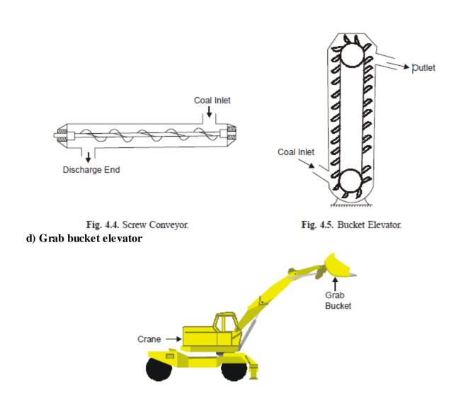
Grab bucket elevator is a device used for both lifting and convey coal on a single rail or track from one point to other
