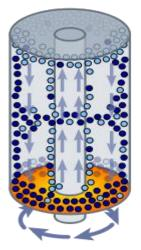
✤ Diagram of the principles of a Zippe-type gas centrifuge with U-238 represented in dark blue and U-235 represented in light blue
