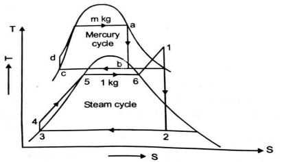
✤ For example, at pressure 12 bar, the saturation temperature of water is 187 °c and mercury 560 °c. Mercury is thus a better working fluid at high pressure range, because at high temperature its vapourisation pressure is low.
