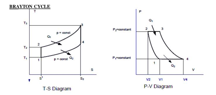
The brayton cycle 1-2-3-4 consists of following four process:
