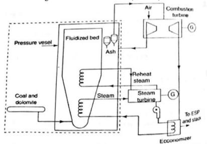
Fig 3.4 Pressurized bubbling fluidized bed combustor (PBFBC)
