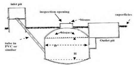
If the gas pressure exceeds the atmospheric pressure (1 bar) and there is no gas extracted from the dome, then the rot substrate squeezed from the reactor into the filled pipe, but often in the pool of counterpoise.
