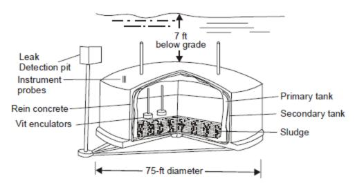
Fig. 11.2. A typical low-level liquid-waste storage tank with double-walled containment.
