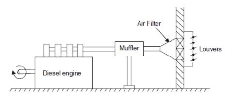
✤ It removes the dust from the atmospheric air and supplies the fresh air to the engine. Super charger,
