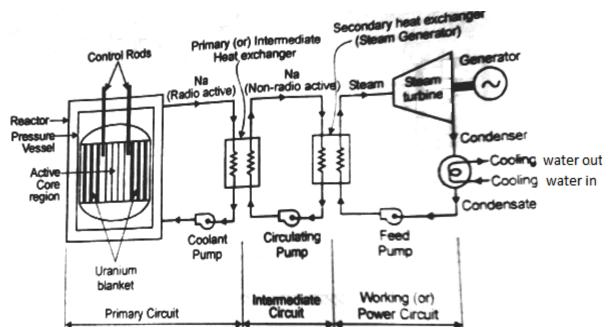
Fig.3.1 Fast breeder reactor power plant (liquid metal cooled reactor).
