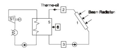
Fig. 2.14. Distributed (Parabolic) Trough Solar Power Plant.
