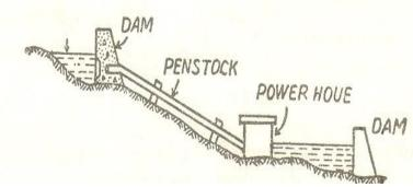
Fig 2.1 High head power plant
