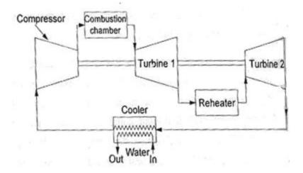
Fig 4-Gas turbine cycle with reheater
