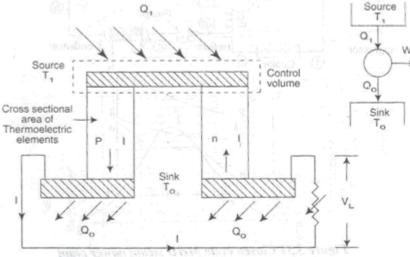
$\clubsuit$  Here applying the first law of thermodynamics to the upper plate as control volume,  $T_i T_o$  will generate a see back voltage. Both junctions are made up of copper element
