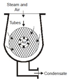
Fig 9.7 central flow condenser
