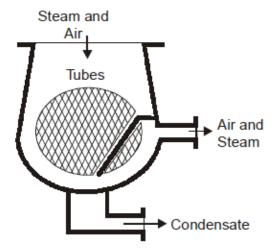
Fig 9.5 Sectional view of down flow condenser
