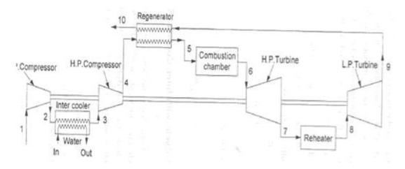
Fig-6-Brayton cycle with inter cooler, reheater and regeneration
