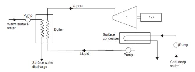
d'Arsonval's original concept in 1881 was that of a closed cycle that also utilizes the ocean's warm surface and cool deep waters as heat source and sink, respectively, but requires a separate working fluid that receives and rejects heat to the source and sink via heat exchangers (boiler and surface con-denser).
