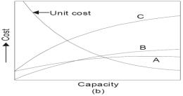
Fig.3.2. shows the variation of various costs of power plant versus its capacity.
