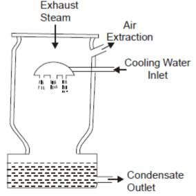
Fig. 9.1 Low level jet condensers
