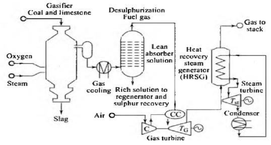
Fig:17.2Integrated Gasifier combined plant
