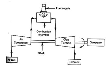
Fig 9.2. open cycle gas turbine power plant
