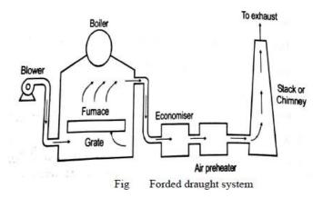
The pressure inside the system is higher than the atmospheric pressure and hence it is also called as positive draught system.
