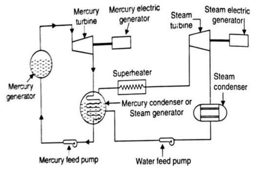
Among these, fluids, mercury is widely used as working fluid because it does not decompose gradually at high temperature.
