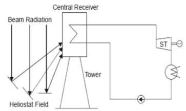
Fig. 5.1 Central Receiver Solar Power Plant.
