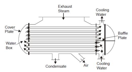
Fig 9.6 longitudinal section view of two pass down-flow condenser
