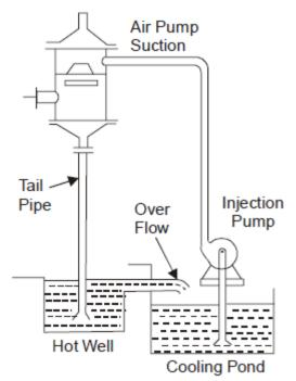
Fig 9.2 High level or Barometric condenser
