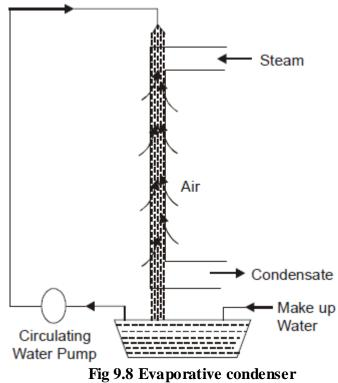
✤ The air is drawn over the surface of the coil with the help of induced fan as shown in Fig. the air passing over the coil carries the water from the surface of condenser coil in the form of vapour.
