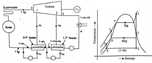
Heat supplied externally in the cycle =  $(h_0 - h_{f6})$ Isentropic work done,= $(h_1 - h_1)+(1 - m_1)(h_1 - h_2) + (1 - m_1 - m_2)(h_2 - h_3)$ Thermal efficiency, =  $\frac{\text{workdone}}{\text{Heat supplied}}$
