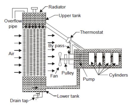
Fig. 12.2 shows forced circulation cooling system
