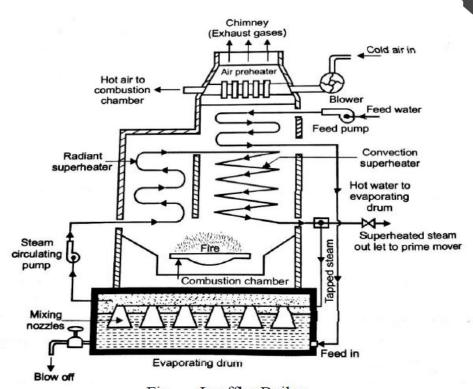
Fig . Loeffler Boiler
