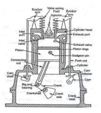
Fig-8- General view of diesel engine
