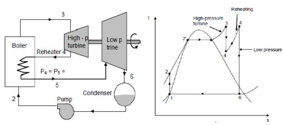
From the figure , the efficiency of the reheat cycle
