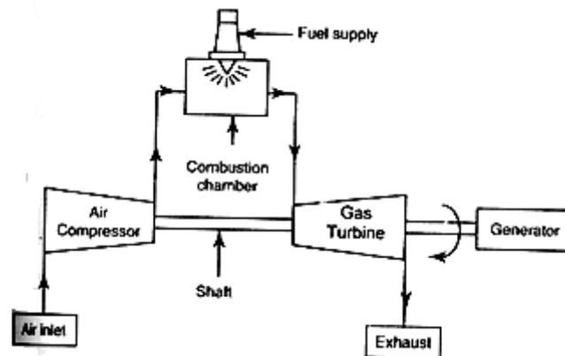
**Fig 9.2. open cycle gas turbine power plant**
