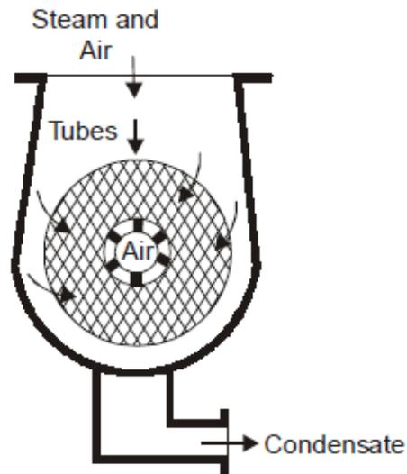
Fig 9.7 central flow condenser
