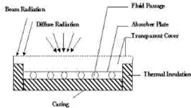
Fig.1 Liquid Flat-plate Collector
