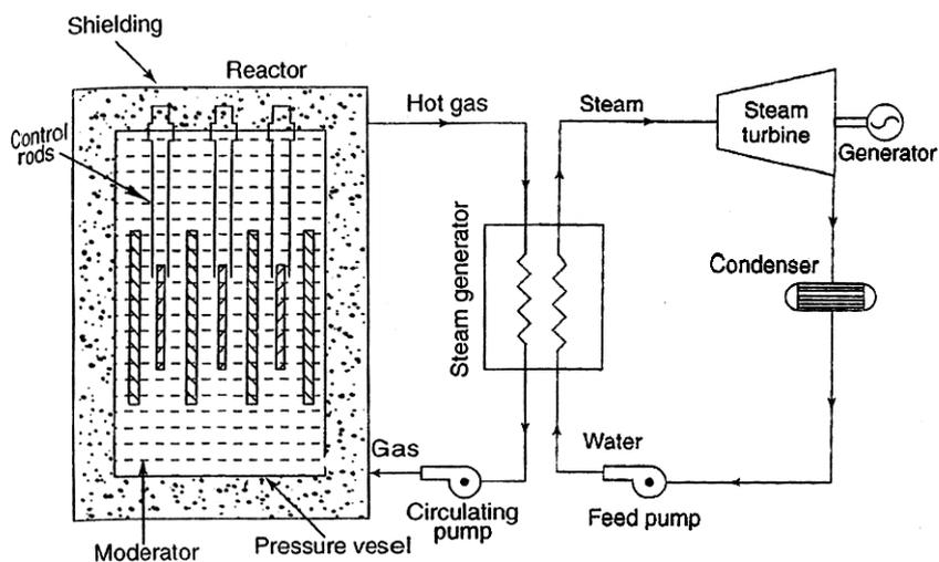
Figure 9.1 Gas cooled reactor
