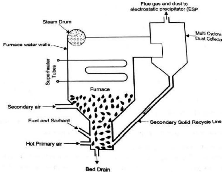
**Fig3.3 Atmospheric circulating fluidized bed boiler**
