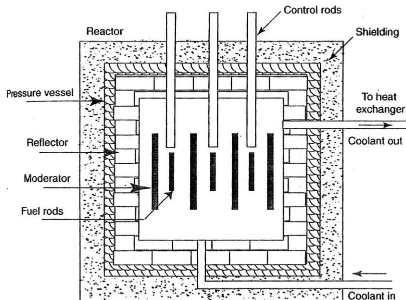
**Fig7.1 Components of Nuclear Reactor.**
