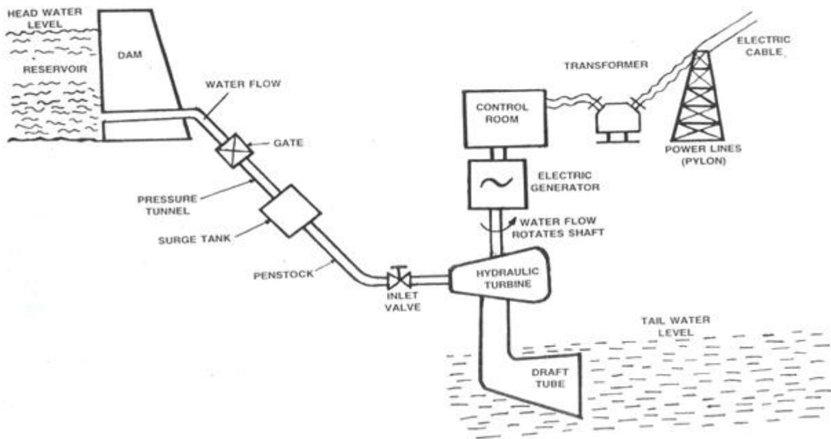
**Fig 1.1 hydro power plant layout**
