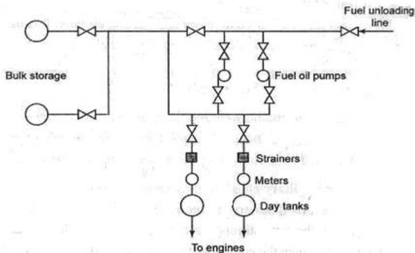
**Fig 11.1 System of fuel storage for a diesel power plant**
