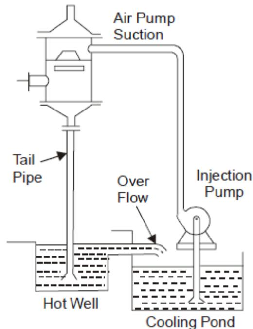
**Fig 9.2 High level or Barometric condenser**
