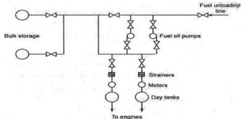
Fig-9- System of fuel storage for a diesel power plant
