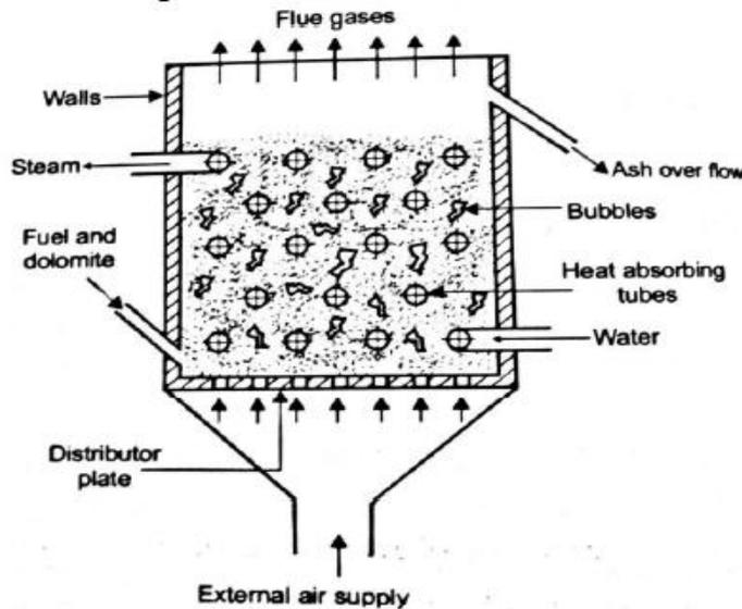
**Fig 5.1 Fluidized bed combustion (FBC) system**
