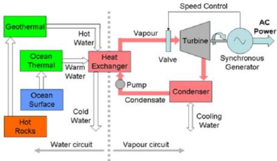
**Fig 4.1 Binary fluid geothermal power system**
