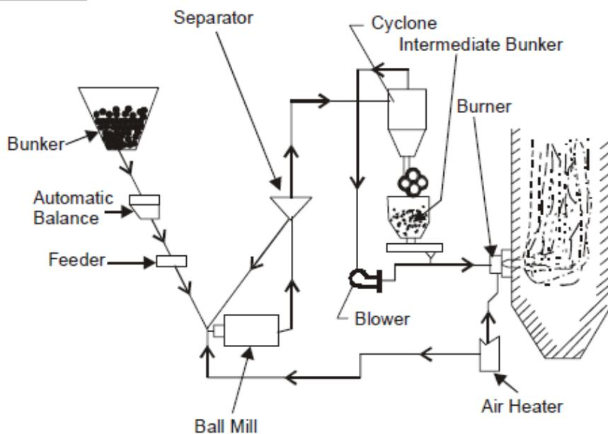
**Figure 16.1 line diagram of ball and race mill**
