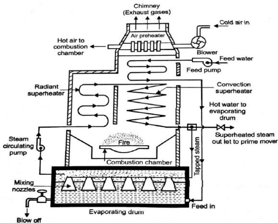
Fig . . Loeffler Boiler
