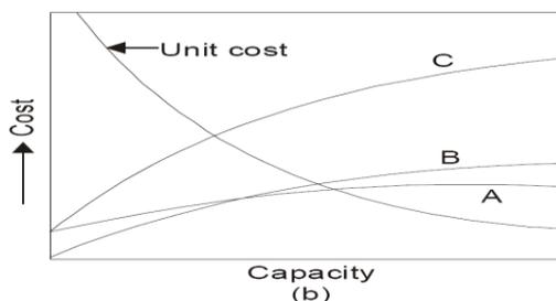
Fig.3.2. shows the variation of various costs of power plant versus its capacity.
