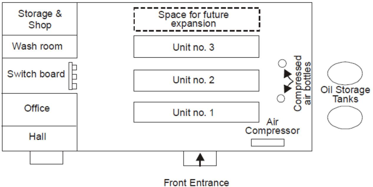
**Fig 5.1 the layout of diesel power plant.**
