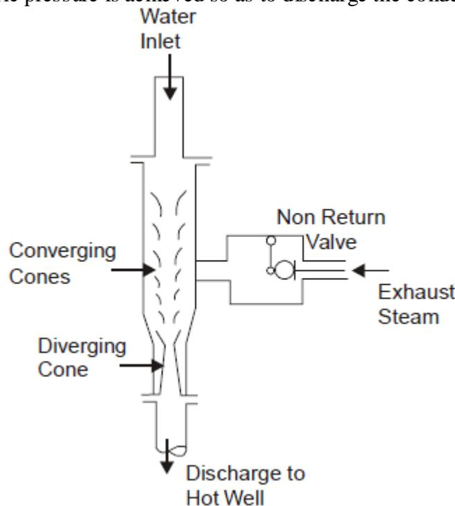
**Fig 9.3 Ejector Condenser**
