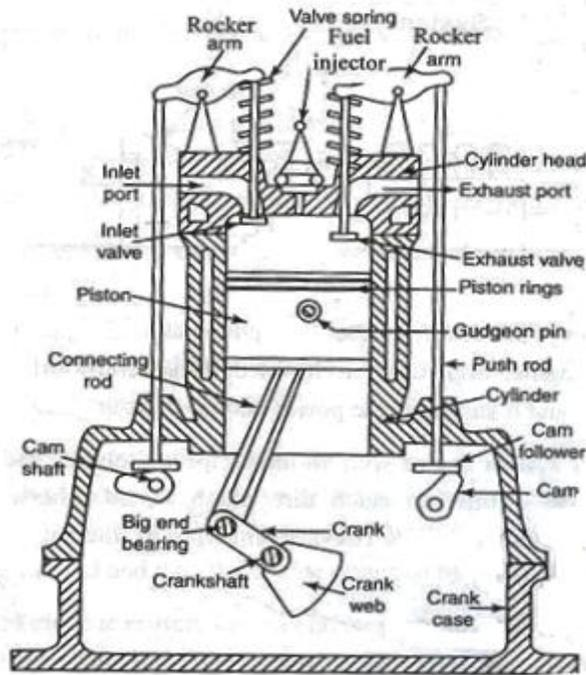
Fig-8- General view of diesel engine
