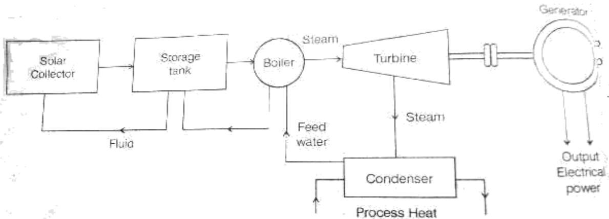
**Fig 5.2 Block diagram of solar power plant**
