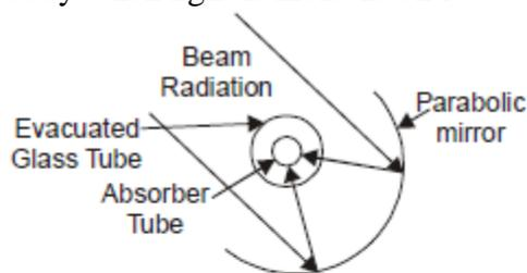
**Fig. 2.13. Distributed (Parabolic) Solar Collector.**
