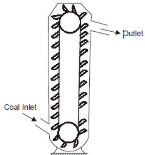
Fig. 4.5. Bucket Elevator.
