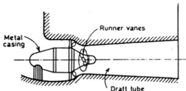
**Fig 1.3 Bulb – type turbine**
