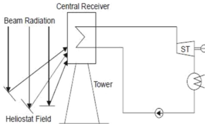
**Fig. 5.1 Central Receiver Solar Power Plant.**
