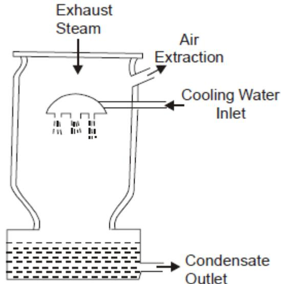
**Fig. 9.1 Low level jet condensers**
