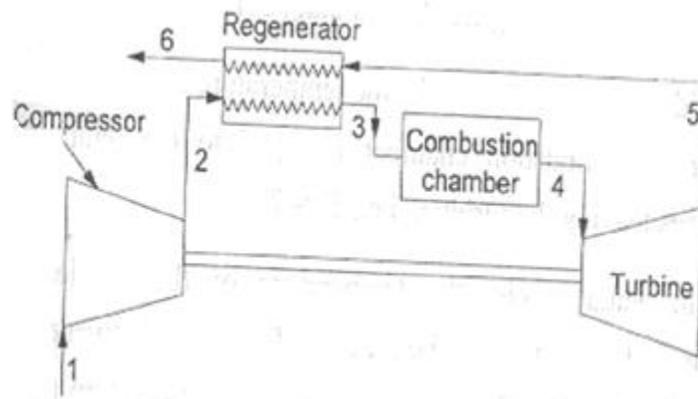
**Fig-1(a) Gas turbine cycle with regeneration**
