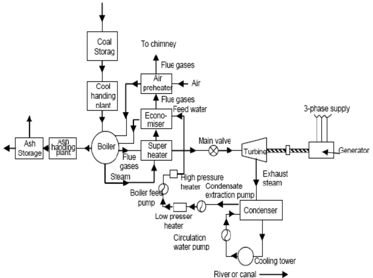
**Fig . Shows a schematic arrangement of a steam power station**
