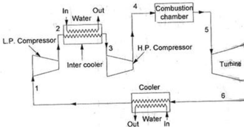
**Fig-3(a)-Gas turbine cycle with intercooler.**
