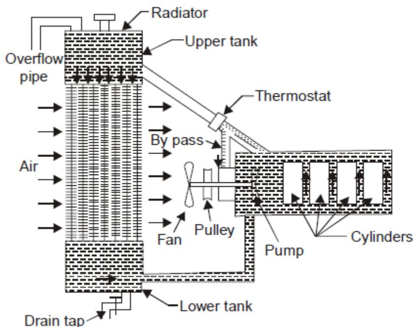
Fig. 12.2 shows forced circulation cooling system
