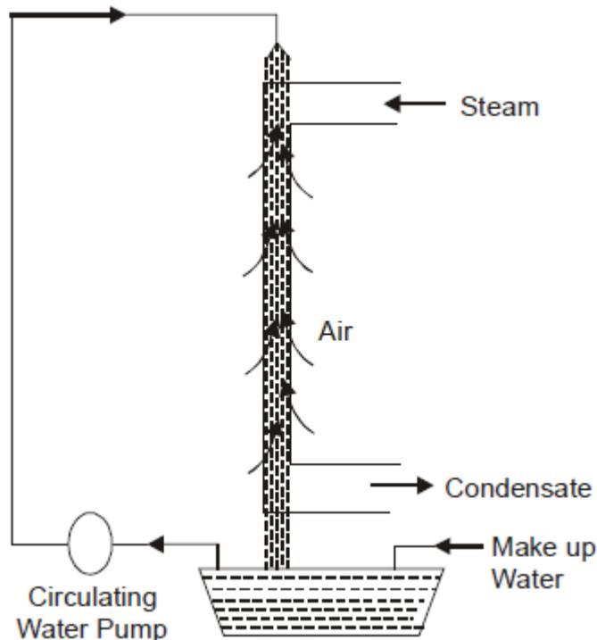
Fig 9.8 Evaporative condenser
