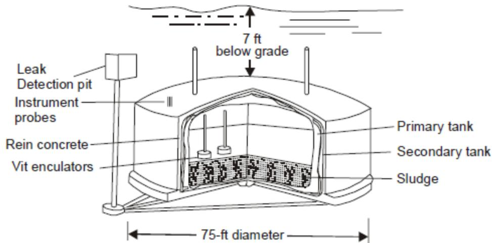
**Fig. 11.2.** A typical low-level liquid-waste storage tank with double-walled containment.
