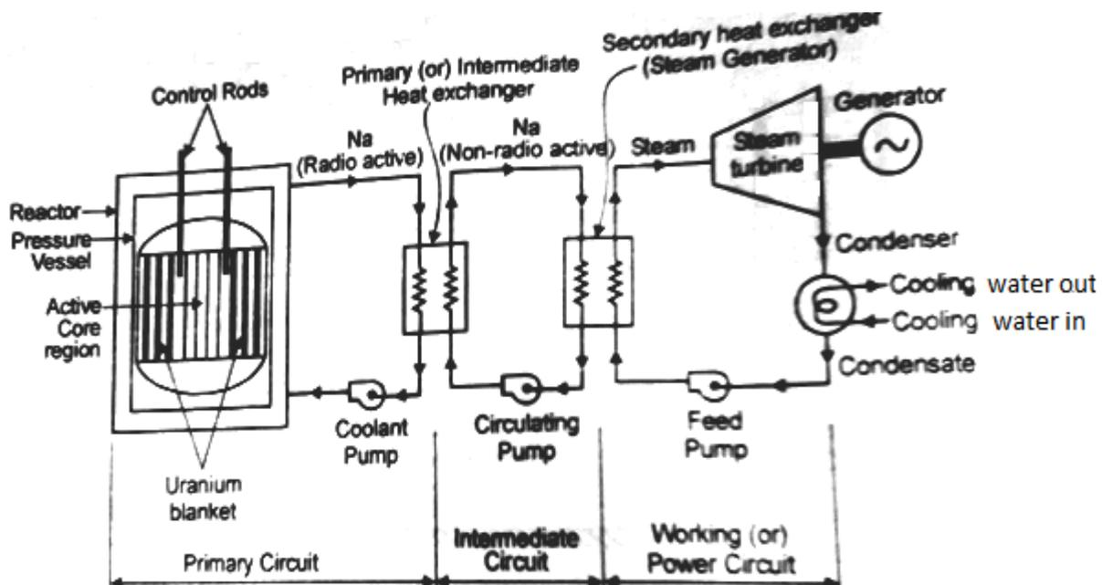
**Fig.3.1 Fast breeder reactor power plant (liquid metal cooled reactor).**
