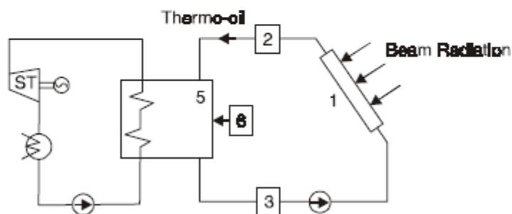
**Fig. 2.14. Distributed (Parabolic) Trough Solar Power Plant.**
