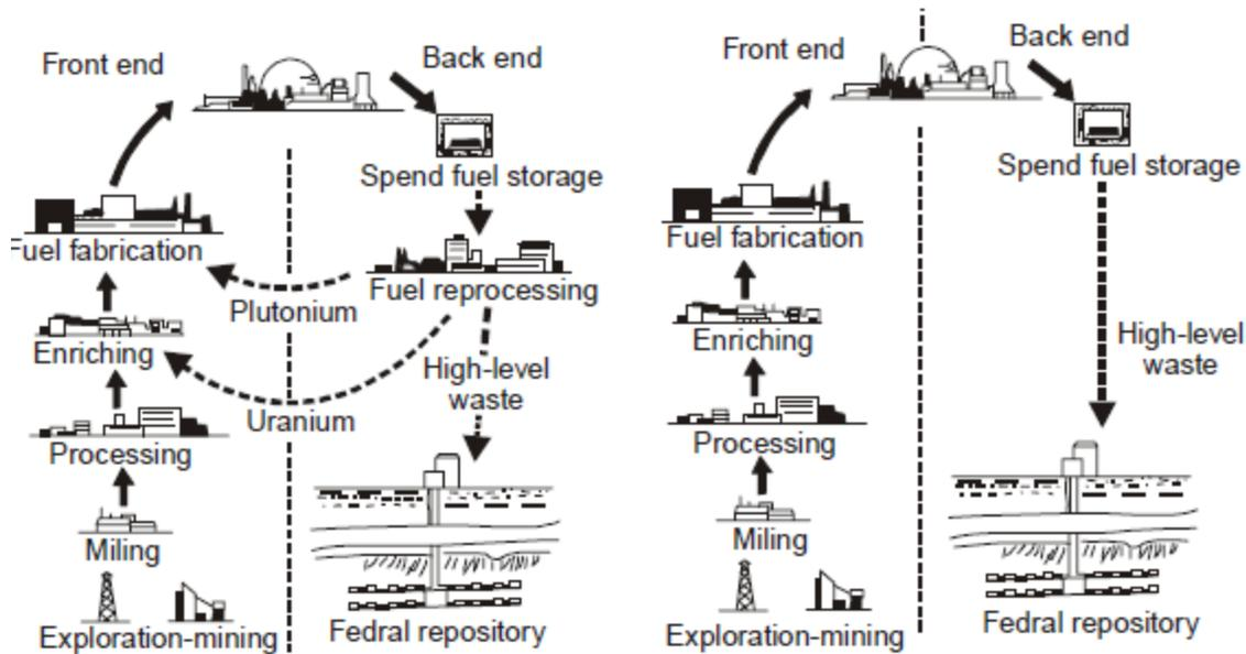
**Fig. 11.1.** A typical nuclear fuel cycle (a) with reprocessing and (b) without reprocessing.
