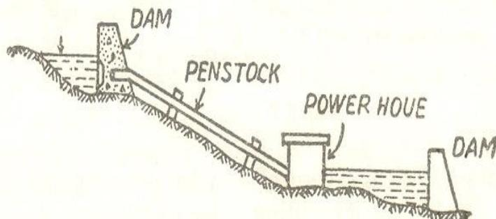
**Fig 2.1 High head power plant**
