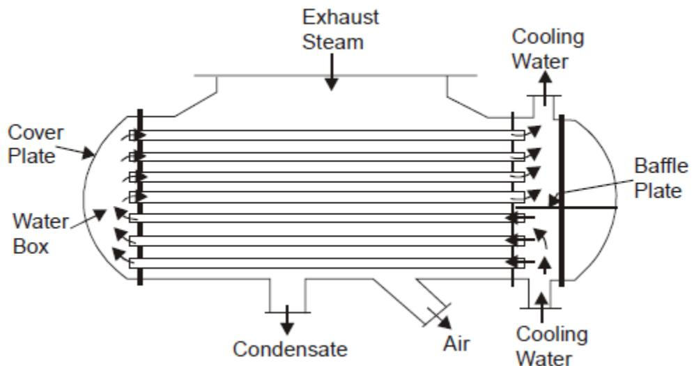
Fig 9.6 longitudinal section view of two pass down-flow condenser
