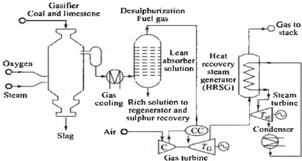
Fig:17.2 Integrated Gasifier combined plant
