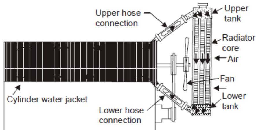
**Fig 12.1 shows a natural circulation cooling system.**
