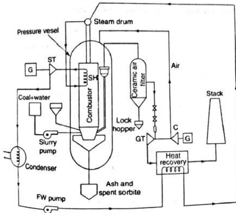
**Fig 3.5 Pressurized circulating fluidized bed combustor (PCFBC)**
