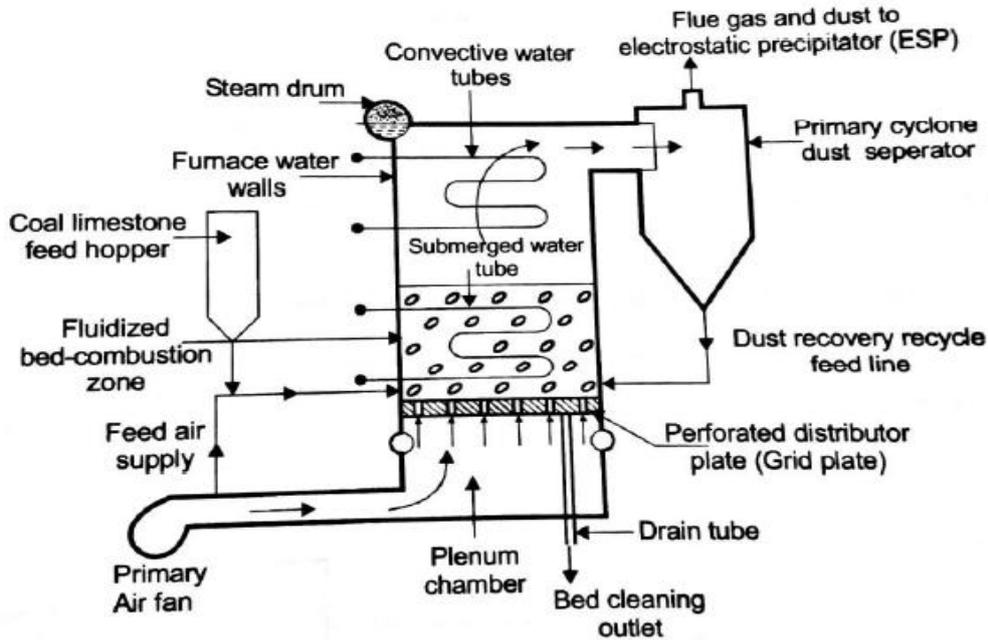
**Fig 3.2 Atmospheric bubbling fluidized bed boiler**
