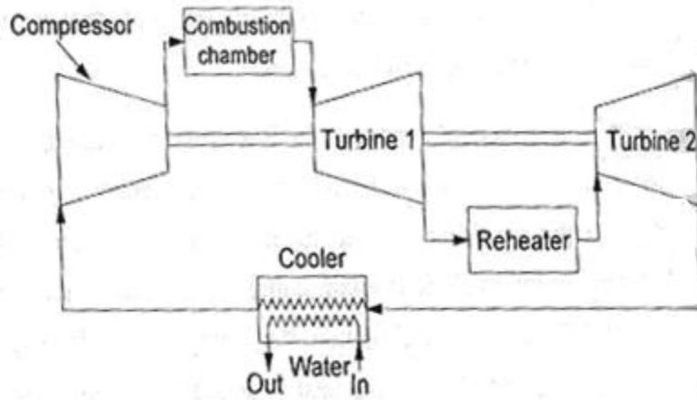
**Fig 4-Gas turbine cycle with reheat**
