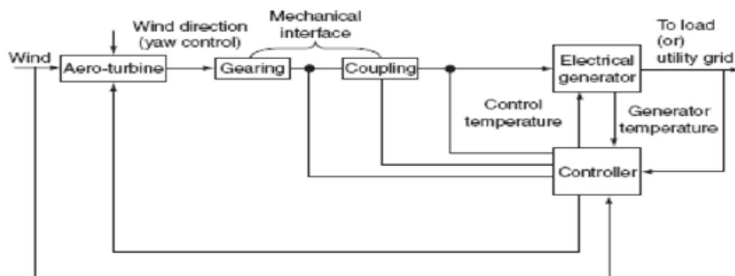
**Fig 2.1 schematic arrangement of wind electric system**
