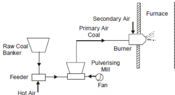
**Fig 17.1 Unit System or Direct System**
